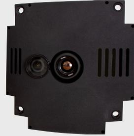
Dial in your mission with our hot-swappable payloads. In 30 seconds, you can change out any camera and put a new one in. All the cameras are housed in identical units allowing them to be interchanged with ease.
